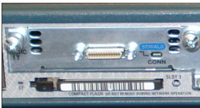
Figura 46. Interface Smart Serial – HWIC-1T.
