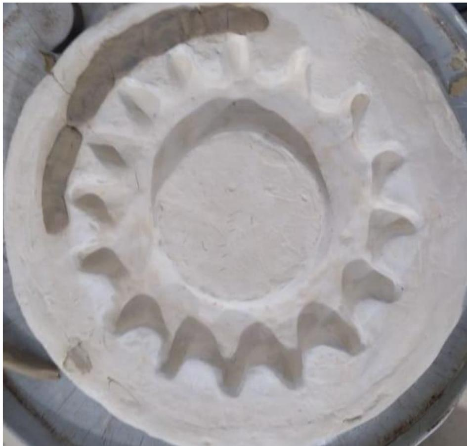
**FIGURA-2** MOLDE PARTE INFERIOR
