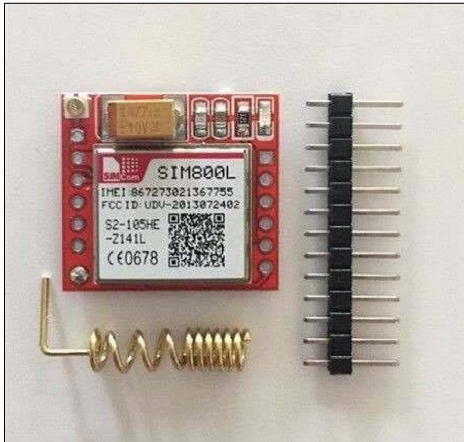
Figura 6 - Arduino Shield GSM SIM800L
